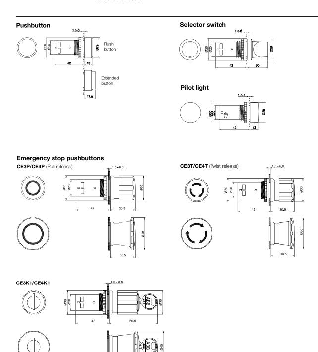
Drilling plans for compact pushbuttons, selector switches, pilot lights and emergency stop pushbuttons. See page  $82\,$
